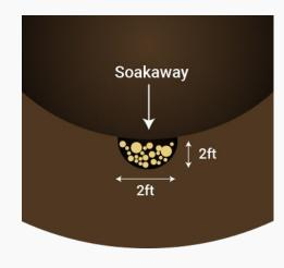
Wrap some membrane over the top of the hardcore/shingle/scalpings and lay some slabs on top to seal the top. You now have a very effective soak-away.
